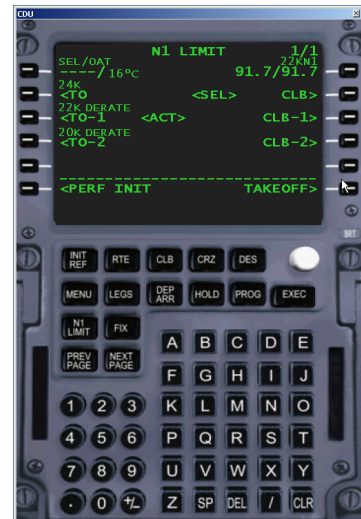
Figure 3 - Setting up for a reduced thrust takeoff
