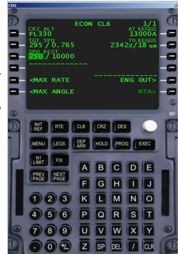
Figure 4 - The CLB page - note the target speed (295/.765M)
