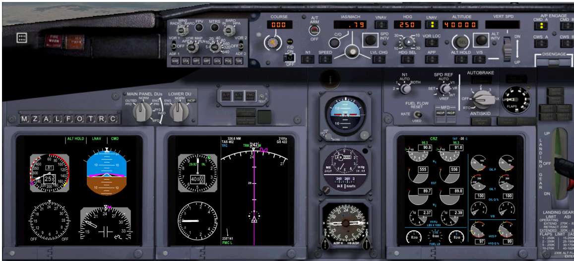
Figure 2 - The EFIS/MAP display
