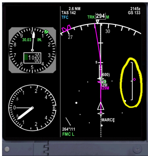
Figure 10 - Path deviation indicator circled on map display
