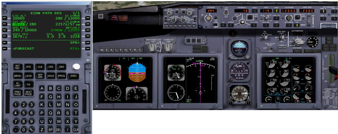
Figure 6 - Initial descent using VS pitch mode - thrust controls airspeed
