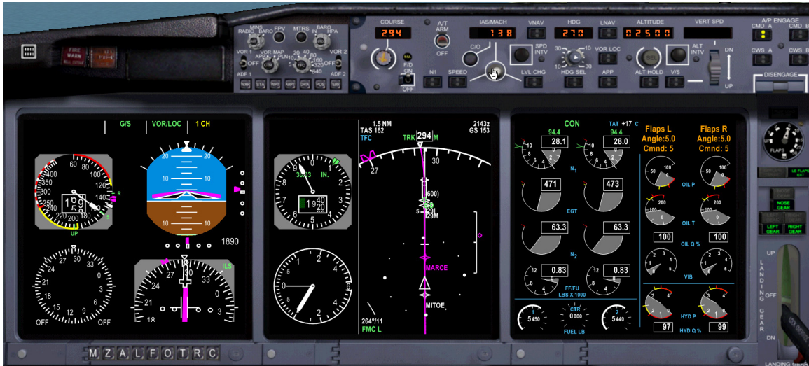
Figure 8 - Slowing to final approach speed
