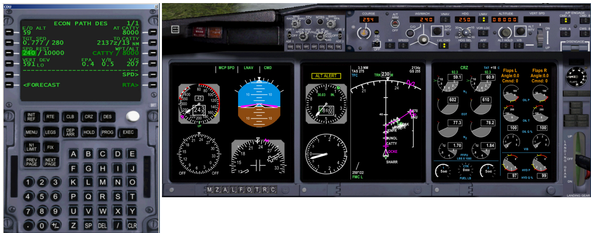
Figure 7 - Descent on arrival using LVL CHG - thrust controls vertical speed
