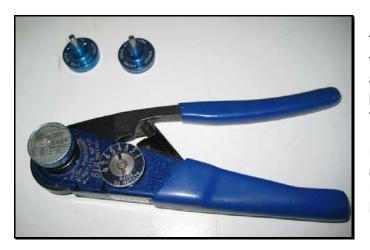
This is an Astro Tool crimper frame part number 615717, and pictured are three positioners (one in the crimper, two in the background). Positioner P/N M22520/2-08 is used for standard D Sub pins and sockets, M22520/2-06 and M22520/2-09 are used for high-density pins and sockets.
