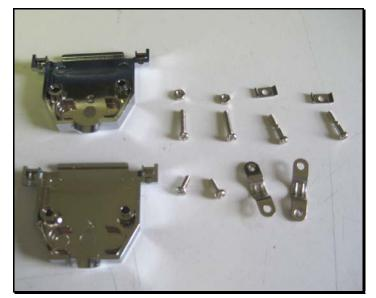
When all wires are inserted, the connector hood can be installed. These are the components of the hood.
