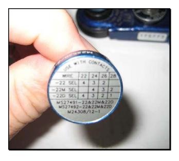
The top of the positioner is labeled with the correct crimp setting for the type of wire that you are using. It is very important to follow this and not over crimp the pin onto the wire. Over crimping always leads to the wire breaking off of the pin.
