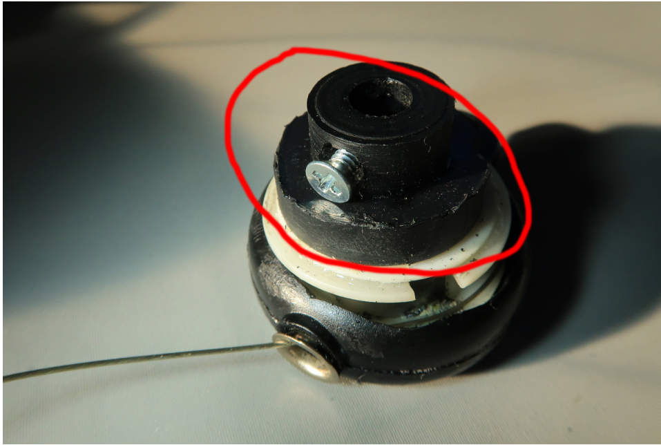
Figure 3: The retractable spring-loaded spool removed from the base of box. Note the screw which is used to secure the spool to the shaft of the potentiometer. Also note that the two-tiered ,black-coloured cylindrical attachment (with the screw). This has been fabricated from ABS plastic and glued to the spool (circled in red).
