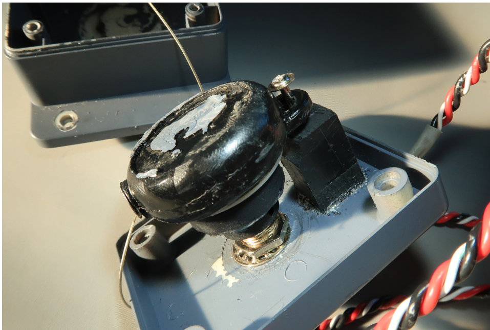
Figure 4: The lid of the box showing the retractable spool secured to the shaft of the potentiometer. The discolouration on the base of the spool is old glue ( from when I dismantled the unit to take photographs ). Note the screw attached to the piece of ABS plastic. This screw helps to secure the spool.
