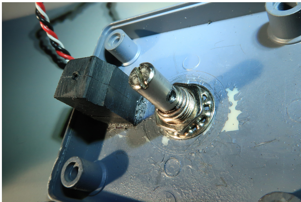
Figure 2: The inside lid of the box with the shaft of the potentiometer secured by a nut a washer. Note the hole that has been carefully drilled into the shaft. This hole aligns with the hole drilled in the side of spool (Figure 3). A screw secures them together to stop the spool from free spooling. The piece of ABS plastic with a small drill hole is also seen .
